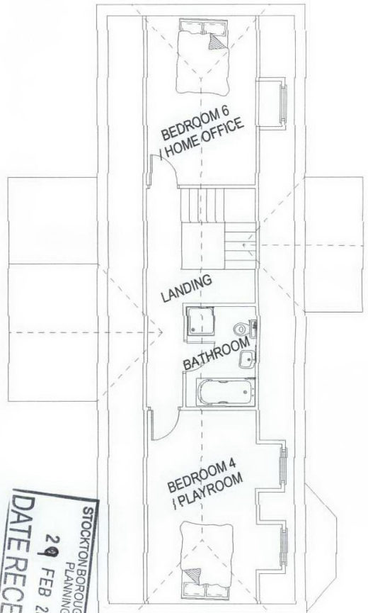
PROPOSED ATTIC FLOOR PLAN ( scale 1:100 )
